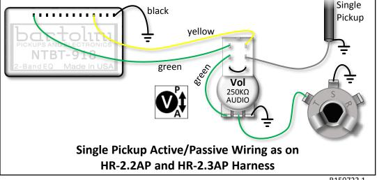
Ground - Connected to preinstalled bare wire. Connect to cavity shield if available. Also ensure bridge is connected to ground.
